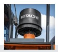
ENGINE AIR PRE-CLEANER An optional, adjustable, rotary pre-cleaner pulls clean air into the engine when working in tough conditions.
