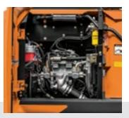
SAME-SIDE FILTERS Engine oil, fuel and hydraulic pilot oil filters are all located on the same side at ground level for easy servicing.
