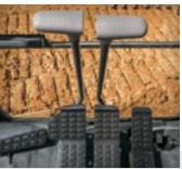
SINGLE-PEDAL PROPEL An optional, hydraulic, singlepedal propel system allows straight-line machine tracking without articulating both hand and foot pedals.
