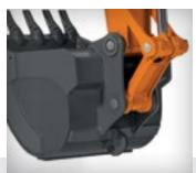
PROTECTED JOINTS Tungsten-carbide-coated surfaces protect the critical bucket-to-arm joint.
