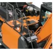
STANDARD HANDRAILS Upperstructure handrails provide added safety when servicing the engine compartment, and a larger hood gives you better engine accessibility.
