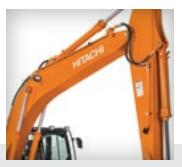
**AUXILIARY LINES** Optional auxiliary hydraulic lines with combination piping increase machine versatilit
