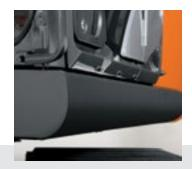
**REINFORCED SIDE FRAMES** Reinforced D-channel side frames provide maximum cab and component impact protection.
